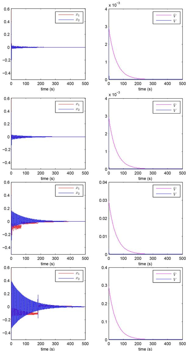
Fig. 3.  $\eta(0) = 0.1\bar{\eta}(0)$ ,  $\eta(0) = \bar{\eta}(0)$ ,  $\eta(0) = 10\bar{\eta}(0)$ , and  $\eta(0) = 100\bar{\eta}(0)$ , system states; Lyapunov function evolutions and their references.
