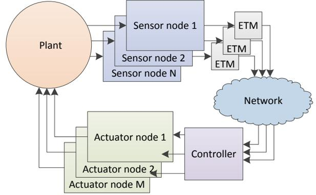
Fig. 1. Networked systems architecture, with decentralized event-triggered mechanism (ETM).
